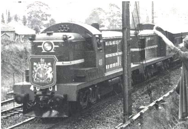
Above: Royal Train at Duffy Ave, Thornleigh, Tuesday 9 February, 1954. Two ALCO class C40 diesel electric locomotives end to end, led by #4001 painted royal blue with yellow trim, on Sydney to Newcastle run.
