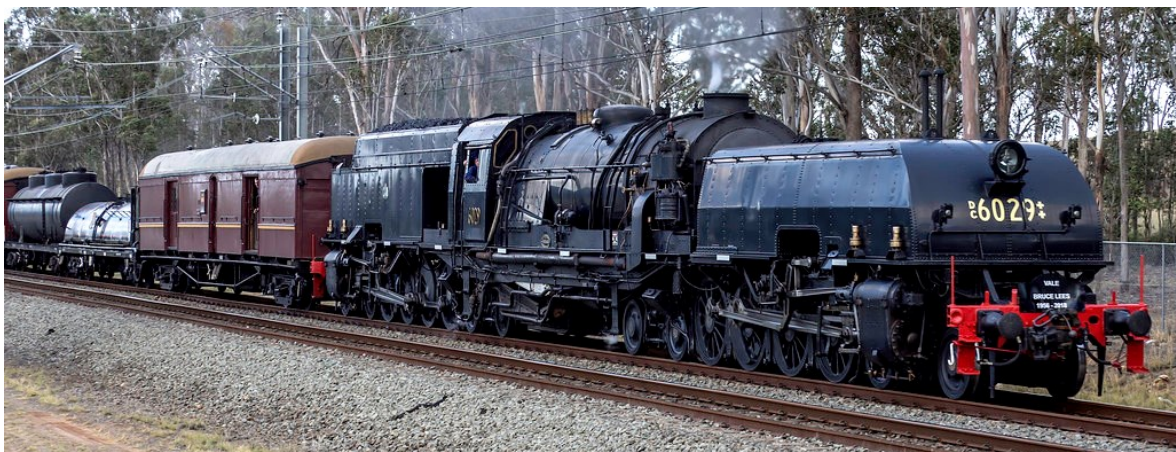
NSWGR AD60 class Garratt locomotive (4-8-4+4-8-4) produced between 1952-1957 in Manchester. These were three-part articulated heavy goods steam locomotives, and were often roaring up the Beecroft line. We could hear them at home and they were very noisy with a load and in the wet. This one #6029 was in service 1954-1972 and was restored and is owned by NSW Rail Museum Thirlmere [Wikipedia; flickr.com]
